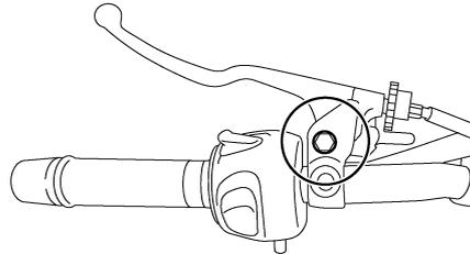
The operation of the brake and clutch levers should be checked before each ride, and the lever pivots should be lubricated if necessary.
