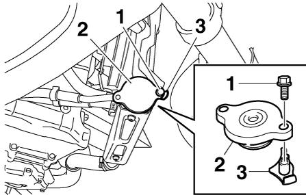
1. Radiator cap retaining bolt
