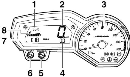
1. Coolant temperature display/air intake temperature display
