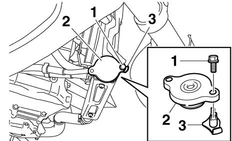
1. Radiator cap retaining bolt
