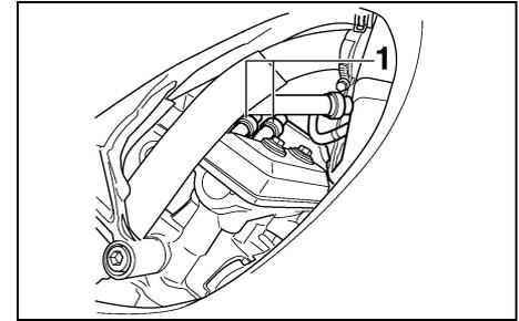
1. Spark plug cap (× 2 on each side)
