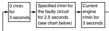
Use this chart to identify what circuit is faulty according to the specified r/min displayed.
