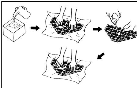
7. Apply recommended oil to the entire surface of the filter and squeeze out the excess oil. The air filter should be wet but not dripping.
