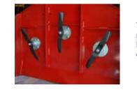
Three blade configuration results in a shorter, more manoeuvrable unit, greater accuracy with height adjustment and less tendency to scalp over rises.
