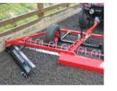
Optional tine bar fitted, seen here with perimeter plough in use to pull in material from the side boards.
