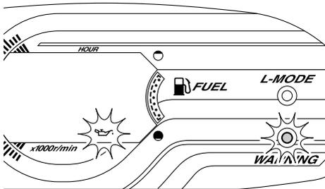
If the oil pressure warning is activated, immediately reduce the engine speed, return to shore, and then check the engine oil level.
