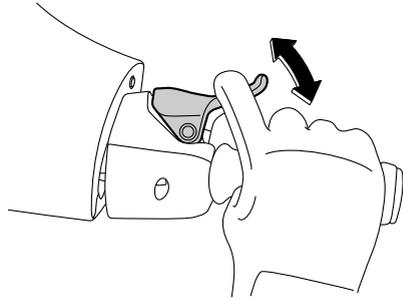
Make sure that there is the proper amount of throttle lever free play when the throttle lever is in the fully closed (idle) position.
