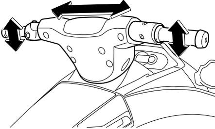
Turn the handlebars as far as possible to the right and left to make sure that the jet thrust nozzle moves as the handlebars are turned, and that there is no difference between the
