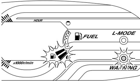
If the fuel level warning is activated, refill the fuel tank as soon as possible. (See page 44 for information on filling the fuel tank.)
