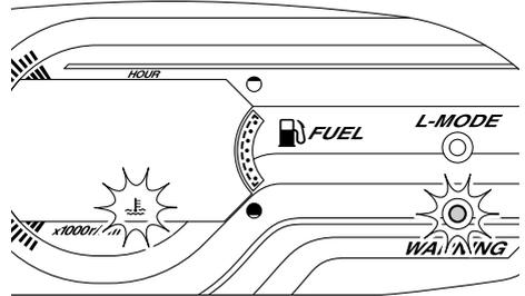
If the engine overheat warning is activated, immediately reduce the engine speed, return to shore, and then make sure that water is being discharged from the cooling water pilot outlet while the engine is running. If there is no discharge of water, stop the engine, and then check the jet intake for clogging. (See page 85 for information on the jet intake.)
