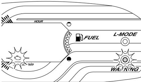
If the check engine warning is activated, immediately reduce the engine speed, return to shore, and have a Yamaha dealer check the engine.
