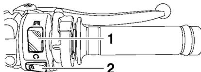
1. Engine stop switch “ $\bigcirc/\text{X}$ ”
