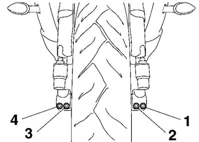
1. Front wheel axle pinch bolt A
