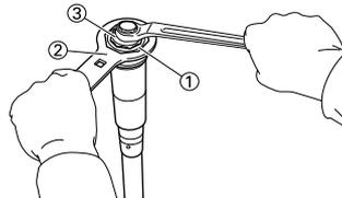
11. After filling, pump the damper assembly "1" slowly up and down more than 10 times to distribute the fork oil.
