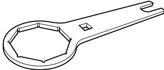
The illustration shows a cap bolt ring wrench, which is a large, open-ended wrench with a hexagonal head and a long handle.                                                                                                                                                                                                                                        |
