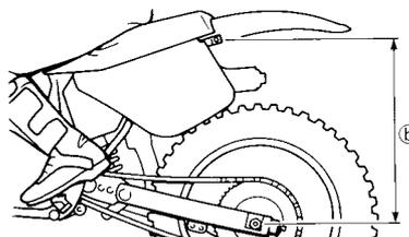
3. Loosen the locknut "1" and make adjustment by turning the spring adjuster "2" to achieve the standard figure from the subtraction of the length "b" from the length "a".
