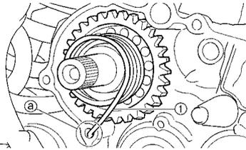
**INSTALLING THE KICK IDLE GEAR**
