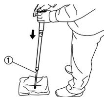
13. Allow the overflowing oil to escape at the hole "a" in the damper assembly.
