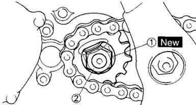
3. Bend the lock washer tab to lock the nut.
