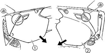
**NOTE:** Put the portion "a" of the flap of the air filter case on the inside of the air scoop.
