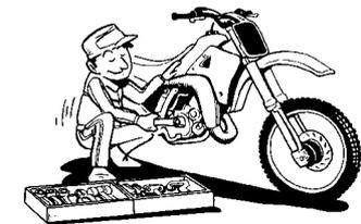
3. When disassembling the machine, keep mated parts together. They include gears, cylinders, pistons, and other mated parts that have been "mated" through normal wear. Mated parts must be reused as an assembly or replaced.
