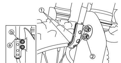
3. Pass the brake hose through the cable guide "1".
