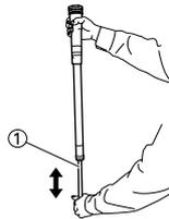
12. While protecting the damper assembly "1" with a rag and compressing fully, allow excessive oil to overflow on the base valve side.
