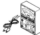
The illustration shows a pocket tester, which is a small, rectangular device with a display screen and several buttons. It is used to inspect the coil resistance, output voltage and amperage.                                                                                                                                                                    |
